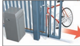
entrapment prevention system reverses gate on contact
