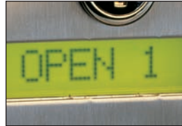
built-in display indicates door/gate has been opened
